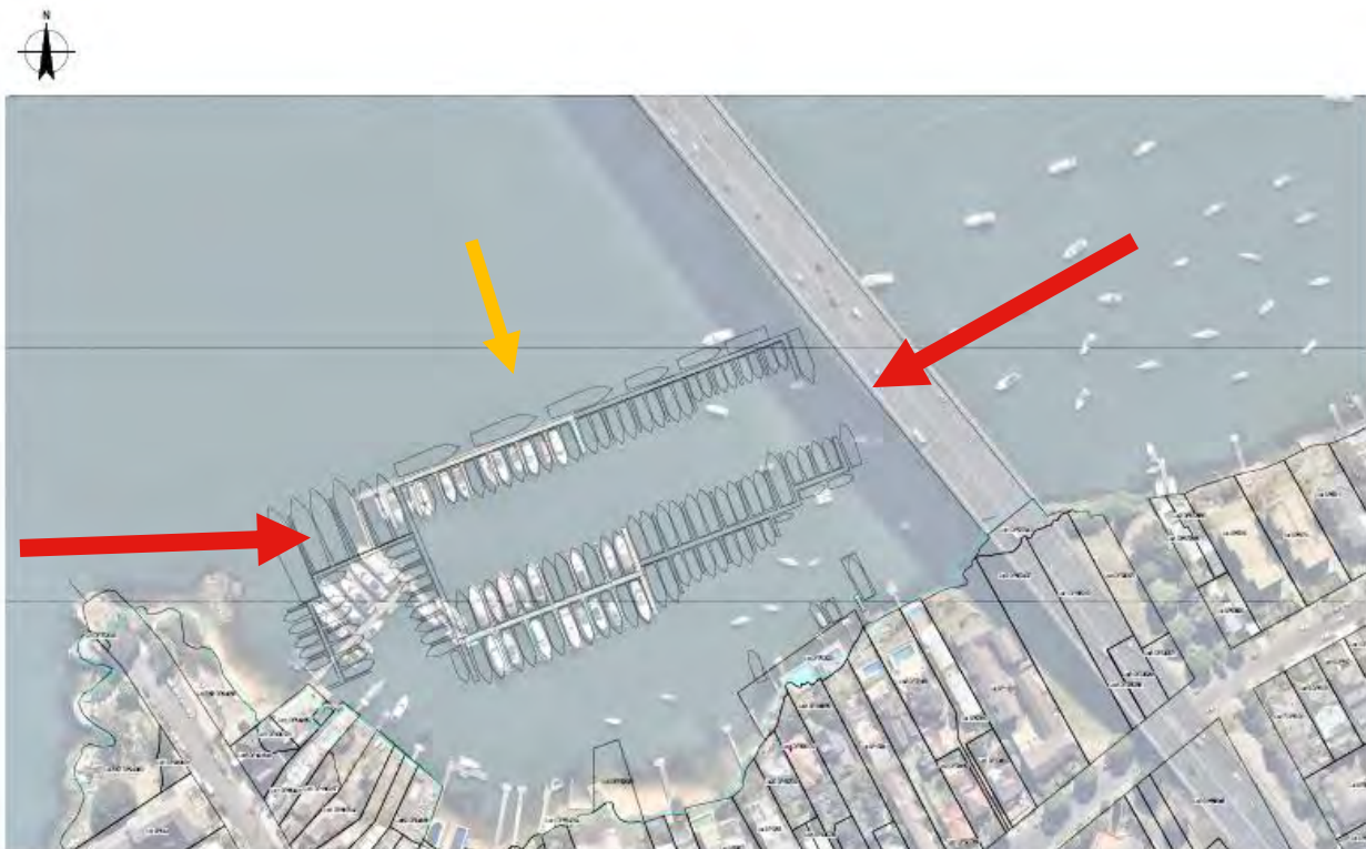
Figure 7-1. Marina wave sheltering actions (dominant wind generated waves (red); dominant boat generated waves (orange))
